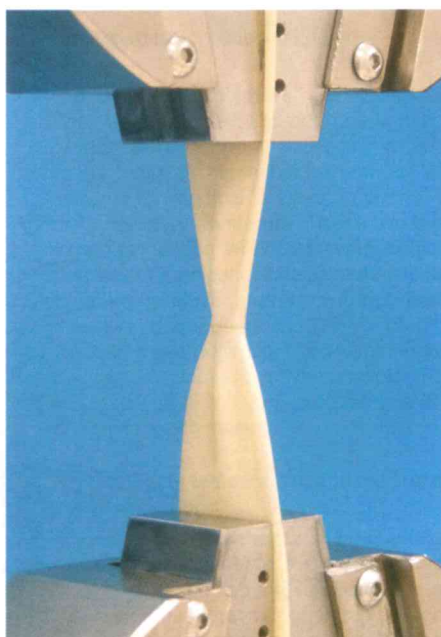
Strength in numbers: Two rubber substrates bonded with new UV adhesive Vitraliot VBB 2N LV show very high bond strength. Image courtesy of Panacol
