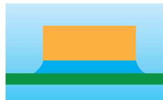
Variations in mounting height of adjacent components (up to 300 percent!)
