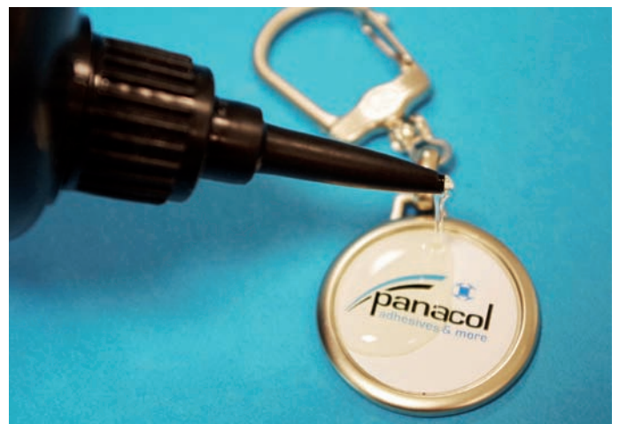
A transparent epoxy resin-based adhesive is applied to create a doming for key rings
